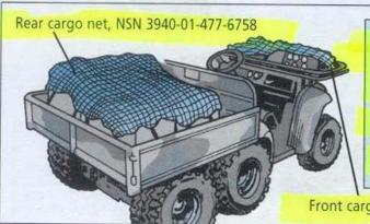
All loads over fifty pounds must be strapped to cargo tie-downs in the back of the vehicle, and the cargo shelf up front. To keep cargo in place, use cargo net, NSN 3940-01-477-6758, for the rear and cargo net, NSN 3940-01-477-7095, for the front.
